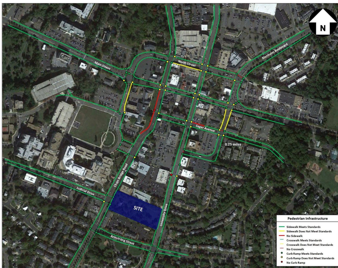
Figure 12: Existing Pedestrian Facilities
