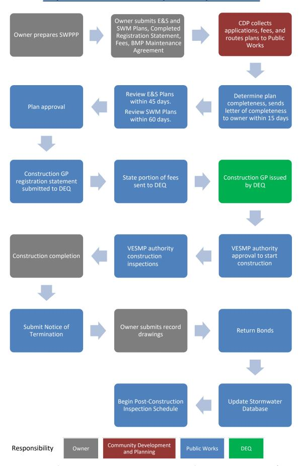
VESMP= Virginia Erosion and Stormwater Management Program, GP= General Permit, DEQ= Department of Environmental Quality, E&S= Erosion and Sediment, SWM= Stormwater Management, SWPPP= Stormwater Pollution Prevention Plan, CDP= Community Development and Planning, BMP= Best Management Practice
