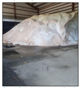
Figure 4. Rock salt is the predominant form of chloride used in liquid and solid forms to control ice formation and snow accumulation.
