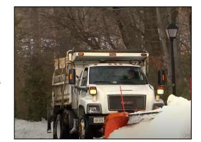
Figure 1. Physically remove as much snow and ice from the infrastructure as possible prior to treatment with chlorides.
