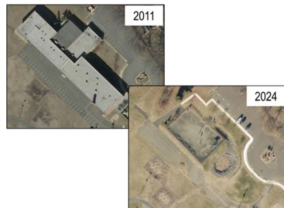
Figure 5. Redevelopment of the Westmore Elementary School into the City Dog Park, demonstrating a reduction in impervious cover and retrofit of previously untreated stormwater runoff
