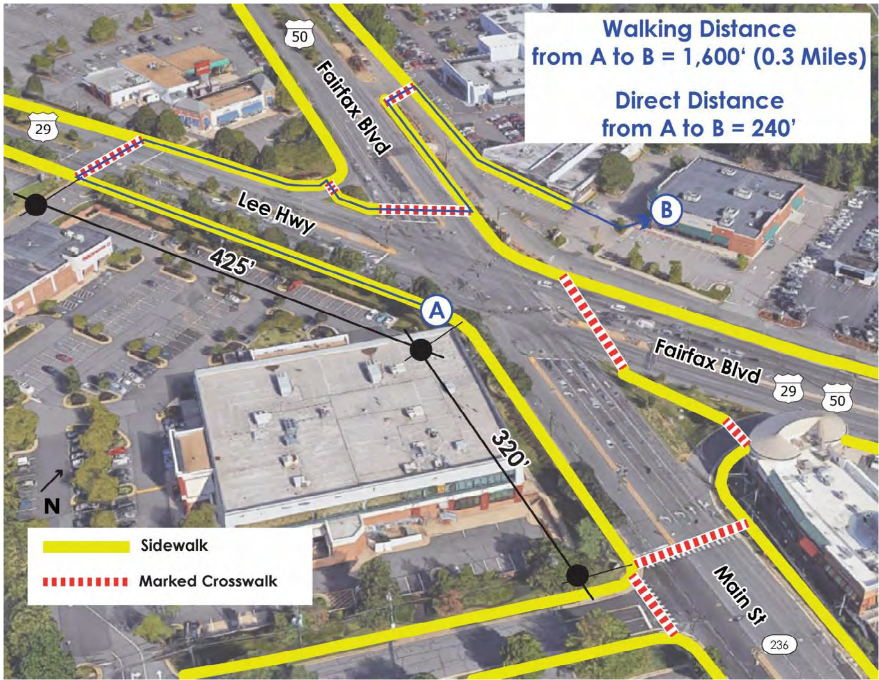
Intersection of Fairfax Blvd and Lee Hwy lacks comfortable crossings on all legs and creates unfriendly pedestrian and bicycle environment
