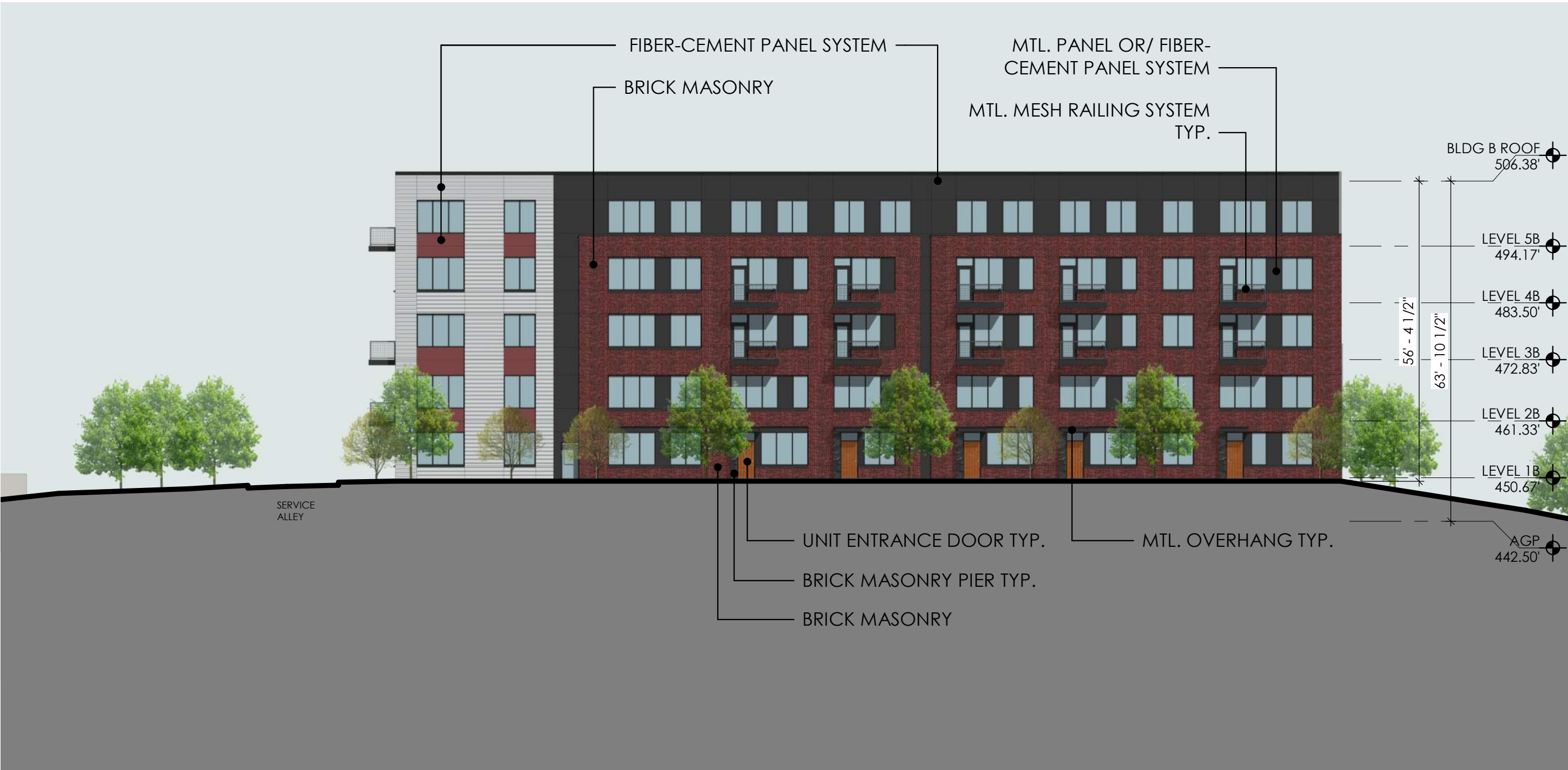
4 BLDG B - WEST ELEVATION AT GREENWAY SCALE: 1" = 20'-0"
