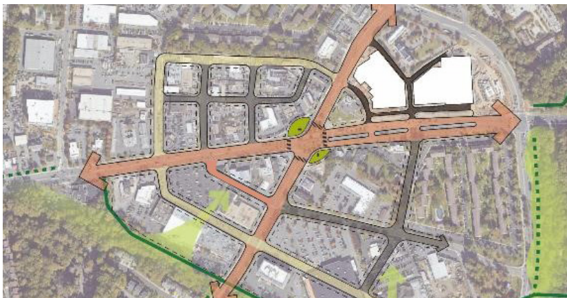
Displaced Left Turn Intersection in Miamisburg, OH. Source: Nearmap
