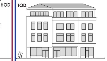
Windows in the HOD are narrow and vertical and there is a higher ratio of wall to window (left). New construction in the TOD can have more window area, and proportion of wall to window can be reduced while still complementing the historic character.
