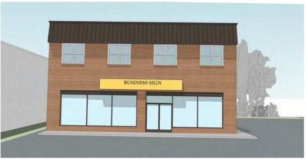
This is an example of an older two-story building with roof modifications that resulted in a heavy metal band at the top of the building.
